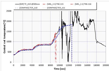
Fig. 5. Control rod temperature evolution
