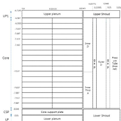
Fig. 1. Node system of COMPASS code
