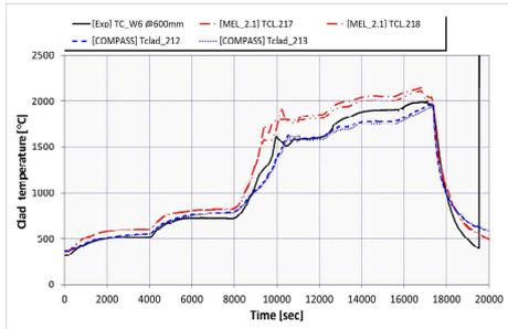
Fig. 4. Clad temperature evolution
