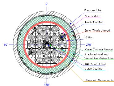
Fig. 2. Cross-sectional view of test bundle
