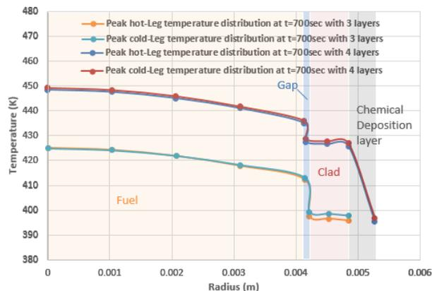
Fig. 11. Peak fuel rod radial temperature profile in hot-leg and cold-leg break, at  $t=700$  sec.
