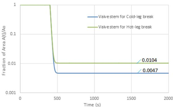
Fig. 2. Valve stem position for the hot-leg and cold-leg break.
