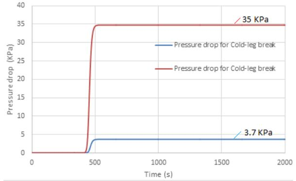
Fig. 3. Debris pressure drop results for hot-leg and cold-leg break
