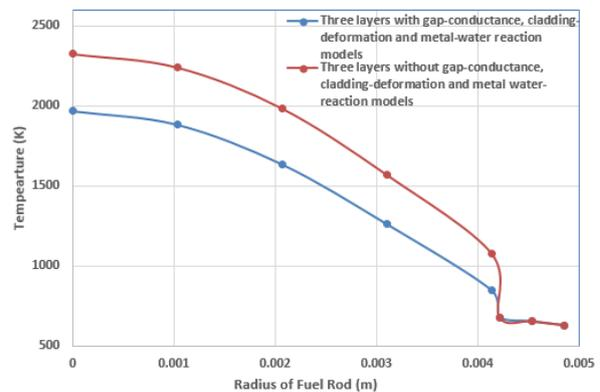
Fig. 5. Temperature distribution with and without gap models in 3 layer case.
