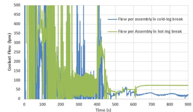
Fig. 9. Flow per assembly in hot-leg and cold-leg break, debris ingress at  $t=400$  sec.
