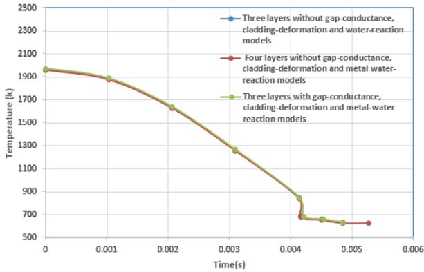
Fig. 6. Temperature distribution with and without gap and deformation models in 3 layer and 4 layer case, after reducing the gap width to 38% of its value.
