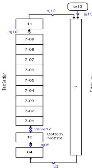
Fig. 1. MARS-KS1.3 model for the test to obtain the pressure drop for debris in cold-leg and hot-leg break
