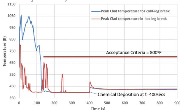
Fig. 10. Peak cladding temperature in hot-leg and cold-leg break, debris ingestion at  $t=400$  sec.
