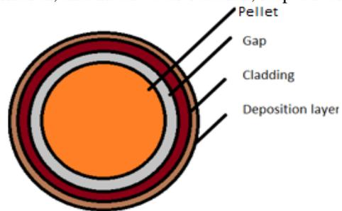
Fig. 4. Modeling of the fourth layer of chemical deposition
