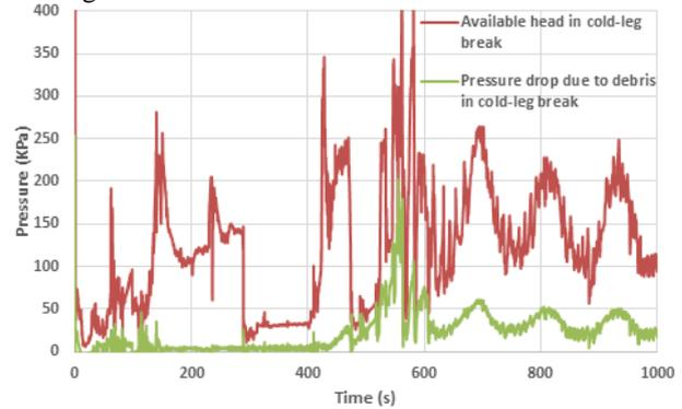
Fig. 7. Comparison of available head and pressure drop due to debris in cold-leg break, debris ingress at  $t=400$  sec.
