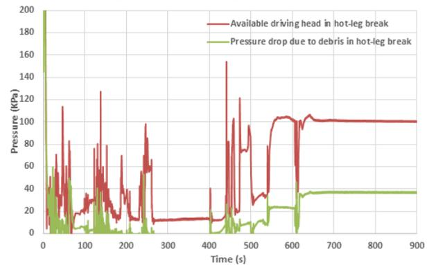
Fig. 8. Comparison of available head and pressure drop due to debris in hot-leg break, debris ingress at  $t=400$  sec.
