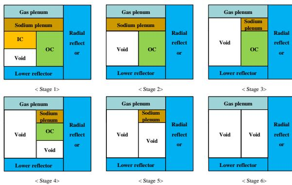
Fig. 6. Axial configurations for the SVR measurements in the BFS-84-1 experiment
