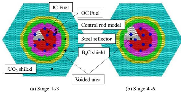
Fig. 5. Radial configurations for the SVR measurements in the BFS-84-1 experiment
