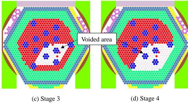
Fig. 4. Radial configurations for stages 3 and 4 SVR measurements in the BFS-109-2A experiment
