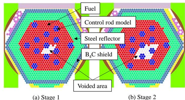
Fig. 3. Radial configurations for stages 1 and 2 SVR measurements in the BFS-109-2A experiment
