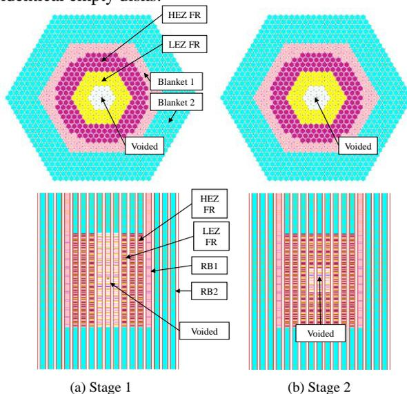
Fig. 1. Radial and axial configurations for stages 1 and 2 SVR measurements in the BFS-75-1 experiment
