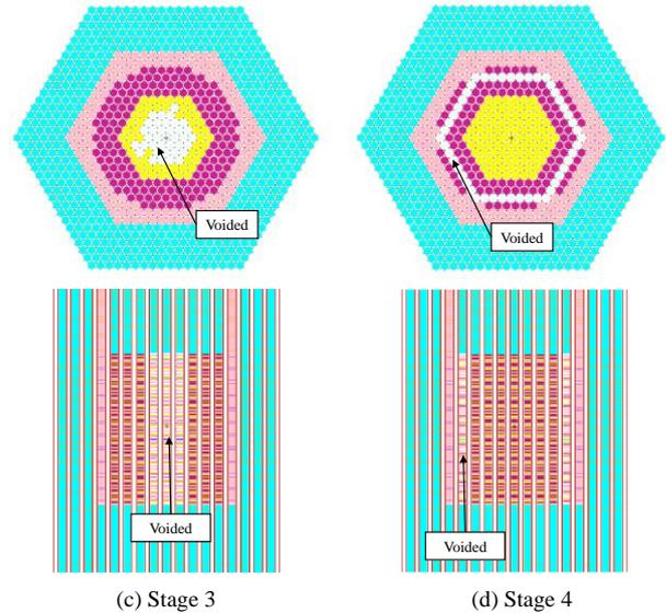
Fig. 2. Radial and axial configurations for stages 3 and 4 SVR measurements in the BFS-75-1 experiment
