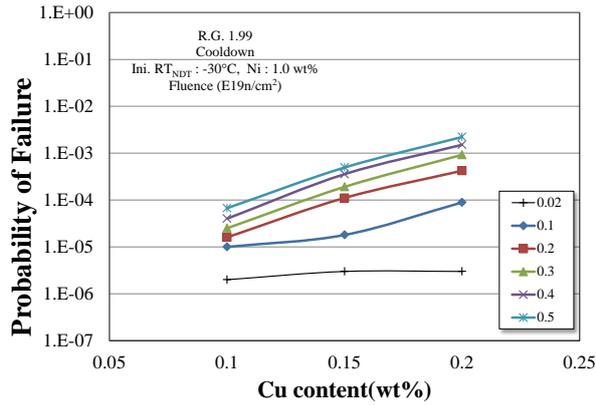
Fig. 4. Effect of Cu content on the probability of failure for cool-down transient.
