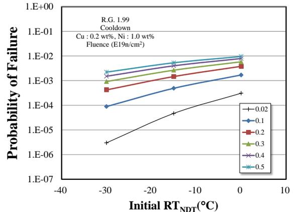
Fig. 3. Effect of initial  $RT_{NDT}$  on the probability of failure for cool-down transient.
