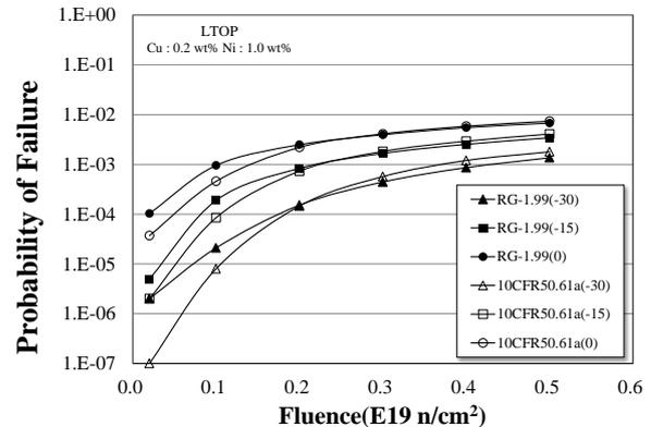
Fig. 2. Comparison of probability of failure between R.G. 1.99 rev. 2 and 10CFR50.61a for LTOP transient.
