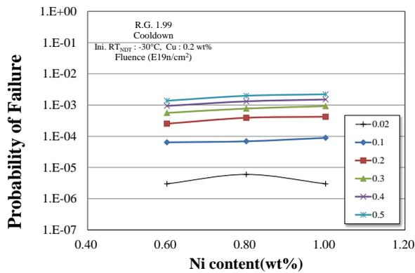
Fig. 5. Effect of Ni content on the probability of failure for cool-down transient.
