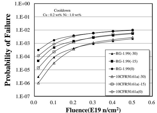
Fig. 1. Comparison of probability of failure between R.G. 1.99 rev. 2 and 10CFR50.61a for cool-down transient.
