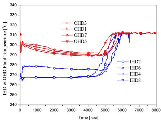
Fig.3. In/Outlet Header Temperature (case 1)
