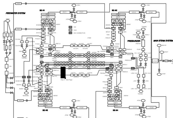
Fig.1. Nodalization Model of CANDU 6 NPP
