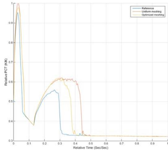
**Figure 4. Difference between the MARS-KS APR-1400 LBLOCA result of radially 50, Axially 50 nodes / radially 17, axially 20 uniformly distributed nodes / radially 17, axially 20 optimized nodes**
