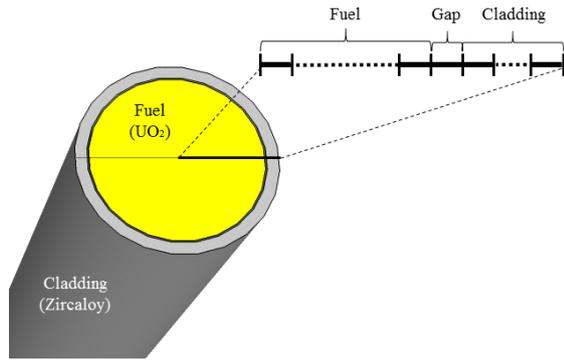
**Figure 1. 1D lumped fuel-cladding system problem concept picture**
