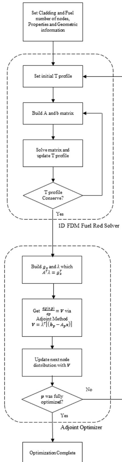
**Figure 2 Calculation Procedure of the Adjoint-based optimization program**
