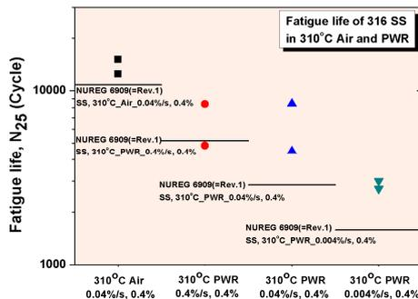
Fig. 2. Fatigue life in 310°C air and PWR environments.
