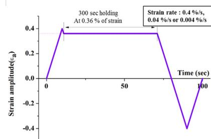
Fig. 1. Strain amplitude curve with sub-peak holding.
