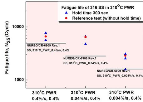
Fig. 3. Fatigue life when the sub-peak holding is applied during 300 seconds.
