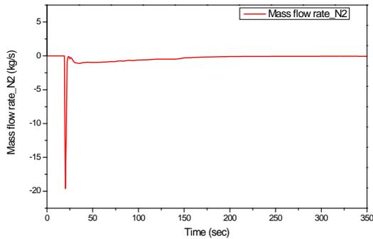
Fig. 3. Mass discharge rate (kg/s) of nitrogen gas.
