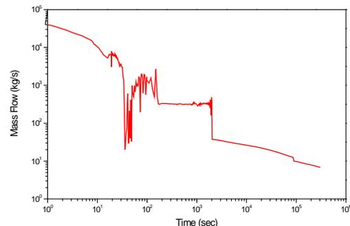
Fig. 1. Mass discharge rate (kg/s) for LBLOCA.
