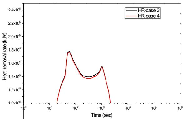
Fig. 8. Comparison of heat removal rate of PCCS conductor of case 3 and 4.
