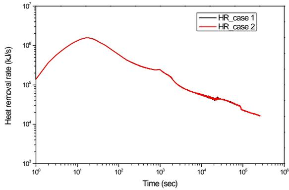
Fig. 6. Comparison of total heat removal rate of thermal conductors of case 1 and 2.
