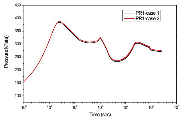
Fig. 5. Comparison of containment pressure transient response of case 1 and 2.
