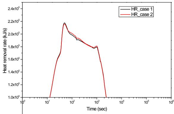
Fig. 7. Comparison of heat removal rate of PCCS conductor of case 1 and 2.
