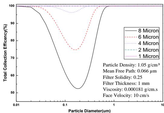
(a) Variable: Fiber Diameter ( $\mu\text{m}$ )
