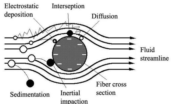
Fig. 2. Aerosol Collection Mechanism of a Single Fiber Filter
