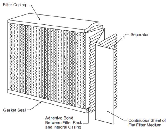
Fig. 1. General design of a Conventional Pleated HEPA Filter at Nuclear Power Plant Air Cleaning Unit
