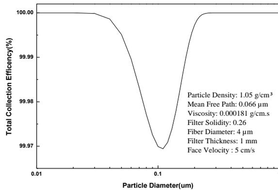
Fig. 5. Theoretical Results of Particle Collection Efficiency for Optimum Design Factor
