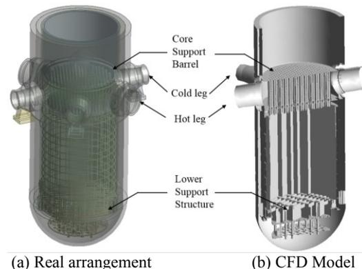
Fig. 1. Schematic of OPR-1000
