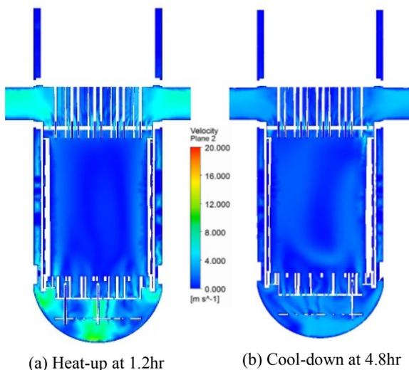
Fig. 3. Velocity distribution at outlet plane
