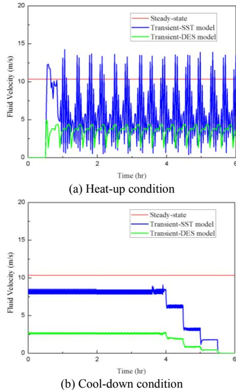
Fig. 4. Comparison of fluid velocities at the center of LSS
