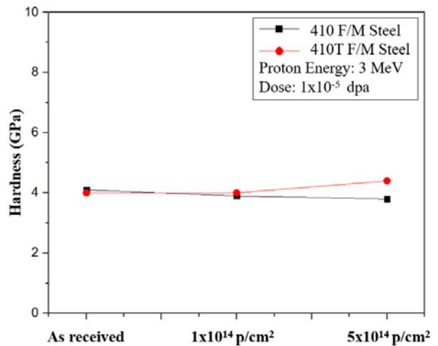
Fig. 2. Effect of proton irradiation on hardness of 410 and 410T F/M steels
