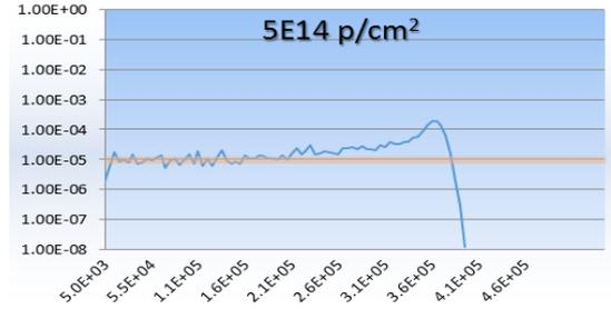
Fig. 1. Penetration depth of 3 MeV proton fluence of  $5 \times 10^{14}$  p/cm<sup>2</sup>
