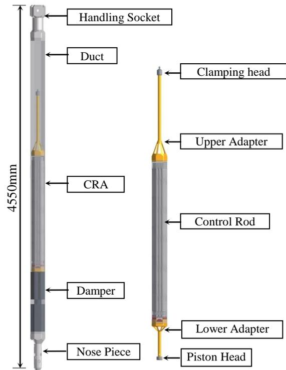
(a) CA (Control Assembly) (b) CRA (Control Rod Assembly)
