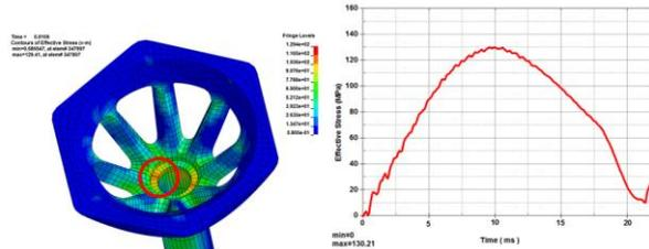
Fig. 10. Maximum stress of Lower adapter of CRA with abnormal conditions
