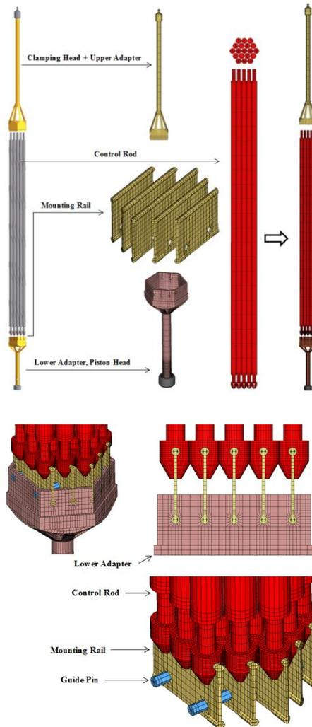
Fig. 4. FE-model of CRA for drop impact analysis
