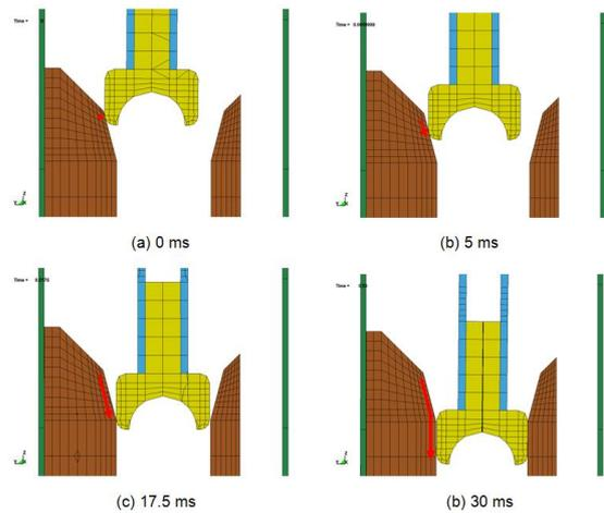
Fig. 8. Dynamic behavior of Piston head of CRA with abnormal conditions
