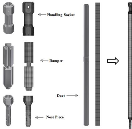
Fig. 3. FE-model of external part of CA
