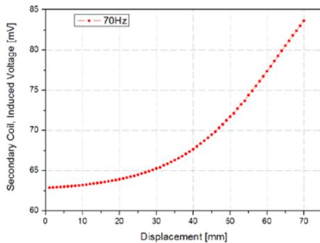
Fig. 5. FEM result of induced voltages
