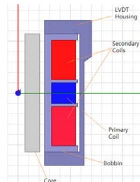
Fig. 3. FEM model of LVDT.
