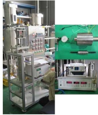
Fig. 6. Experimental setup of proto-type large LVDT.
