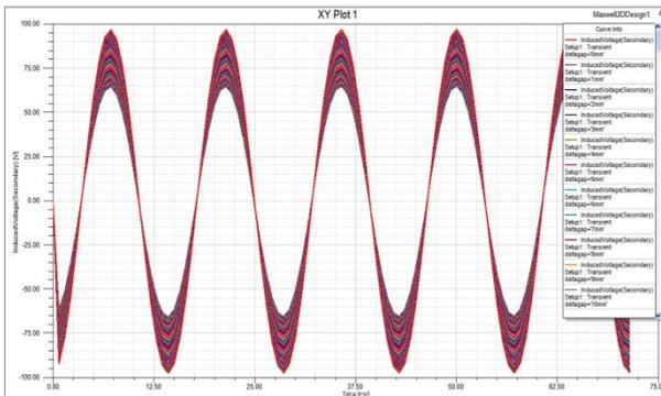
Fig 5 shows summarized induced voltages from secondary coils when the core moves up and down from the center of LVDT. As a result, it is shown that the linearity of the LVDT have a good agreement between 0[mm] and  $\pm 70$ [mm].
