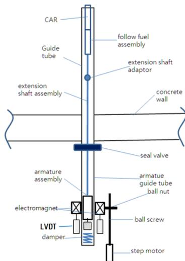
Fig. 1. Schematic of BMCARDM.
