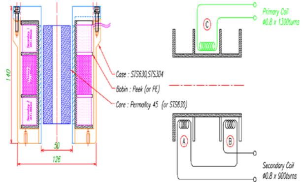
Fig. 2. A detailed view of proposed large LVDT for control rod sagging measurement system.
