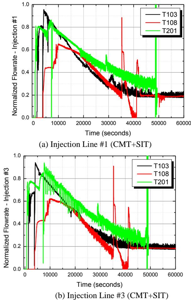
Figure 6 Comparison of injection flowrates.
