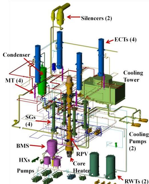
Fig. 1 Schematics of the SMART-ITL.
