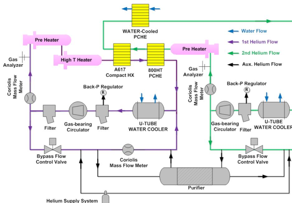
Fig. 1. P&ID of Helium Experimental Loop
