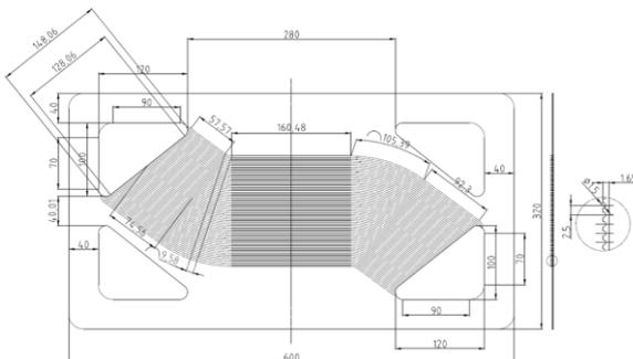
Fig. 2. Stack of Alloy617 Compact Heat Exchanger
