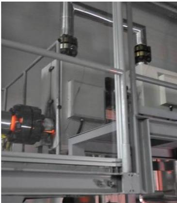
Fig.5 Alloy617 Compact Heat Exchanger during Very High Temperature Condition
