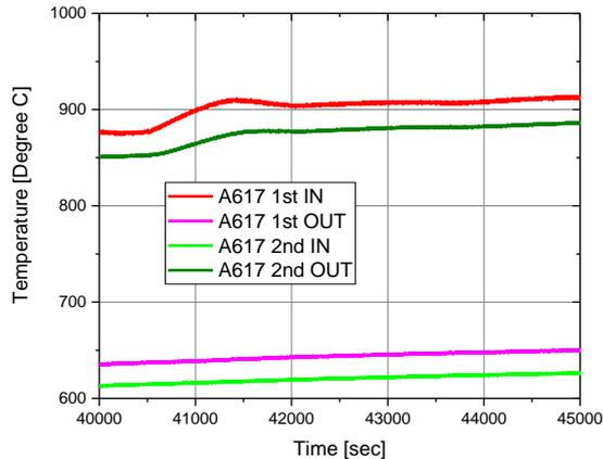
Fig. 4 Temperature Histories of Inlet & Outlet Temperatures of Alloy617 Heat Exchanger
