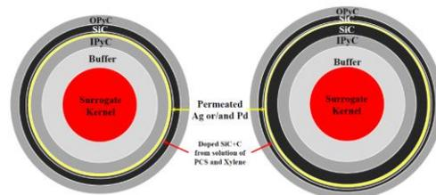
Fig. 1. Schematic illustrations of two kinds of the spherical diffusion couple.
