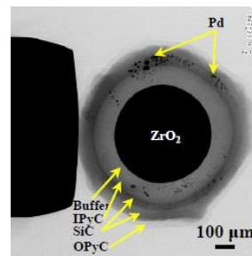
**Fig. 3.** X-ray micro-tomography images showing of the presence of palladium between two layers of SiC and the distribution of pockets of palladium in a H5 particle.
