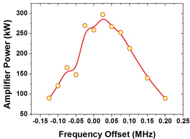
Fig. 4. Amplifier power as a function of frequency offset at the RFQ operating frequency (25.96 MHz).
