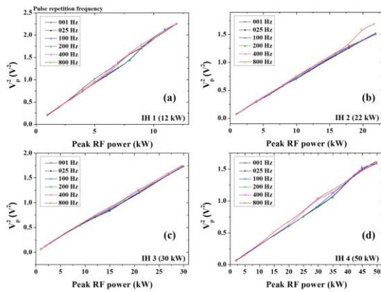
Fig. 3. Measured RF pickup loop voltages in the IH tanks versus peak RF power up to their full power.
