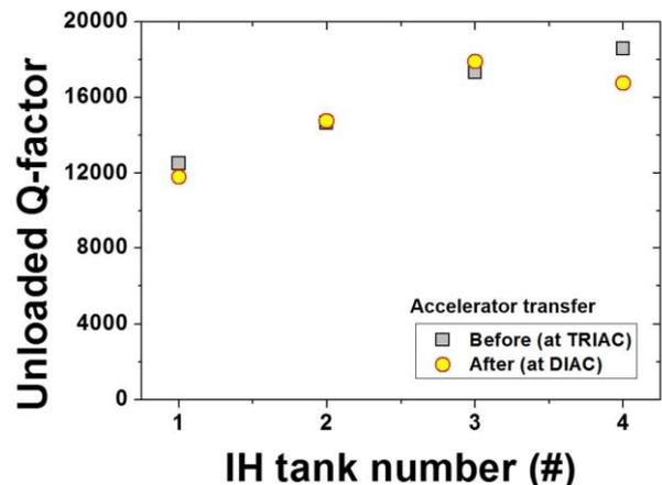
Fig. 2. Measured Q factors of the IH cavities before and after the linac transfer.
