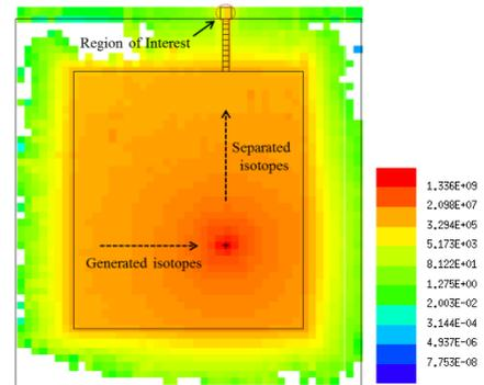
Fig. 1. Dose map of residual radiation in pre-separator room without safety shutter
