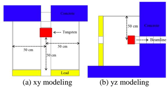
Fig. 5. Modified safety shutter device in pre-separator
