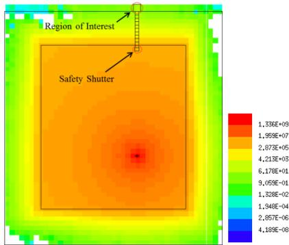
Fig. 3. Dose map of residual radiation in pre-separator room with safety shutter
