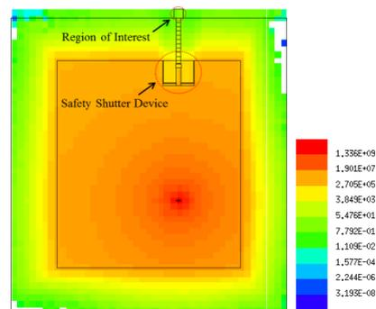
Fig. 6. Dose map of residual radiation in pre-separator room with proposed safety shutter device
