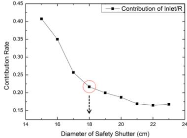
Fig. 2. Contribution rate from beamline inlet to ROI according to diameter of shutter
