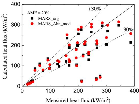
Fig. 10 Comparison of heat flux with Purdue-PCCS in same location (AMF=20%)
