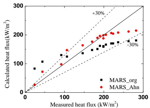
Fig. 8 Comparison of heat flux with JAEA-PCCS in same location
