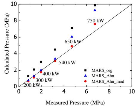
Fig. 6 Comparison of steam generator pressure in PASCAL
