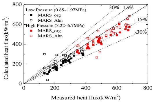
Fig. 3 Comparison of heat flux with PASCAL in same location (Ahn model)
