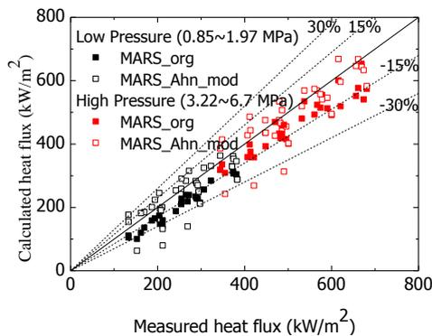
Fig. 5 Comparison of heat flux with PASCAL in same location (modified Ahn model)
