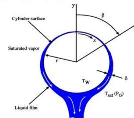
Fig. 1 Film condensation modeling at the outer wall of horizontal cylinder[1]
