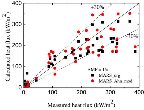
Fig. 9 Comparison of heat flux with Purdue-PCCS in same location (AMF=1%)
