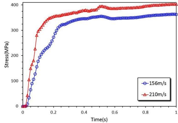
Fig. 5 Stress distributions of liner plate at connector
