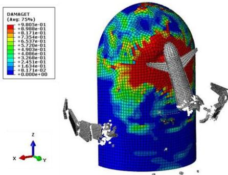
Fig. 3 Damage distribution of concrete
