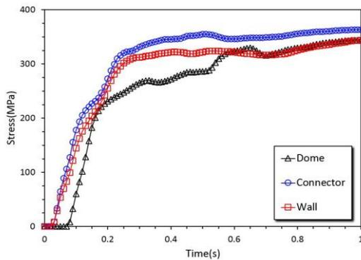
Fig. 4 Stress distributions of liner plate at each location
