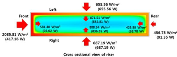
Fig. 2. CFD analysis result: temperature distribution at the outlet cross-section of the riser duct
