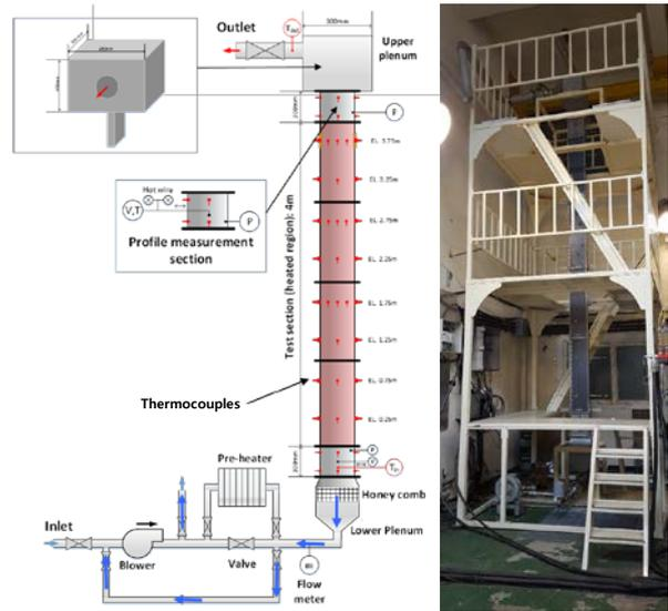
Fig. 3. The schematic diagram (left) and picture (right) of the SNU experimental facility
