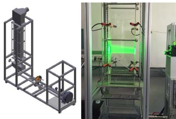
Fig. 4. The design of natural circulation visualization test facility (left) and its experiment (right)
