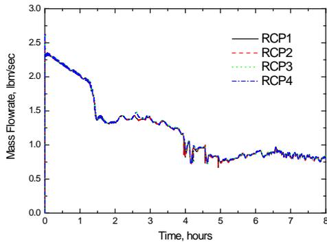
Fig. 4 RCP Seal Leakage
