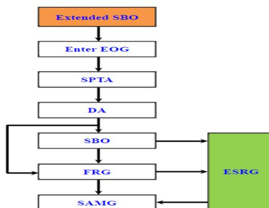
Fig. 1 Schematic diagram for ESRG
