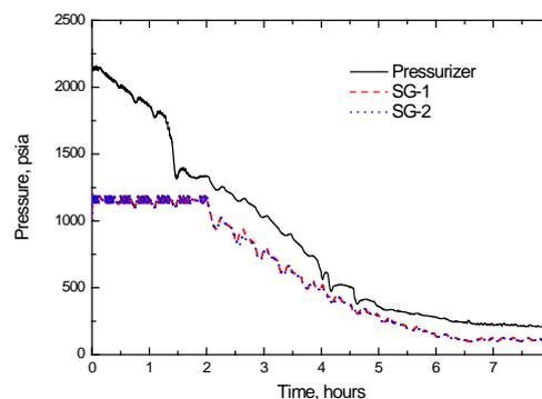
Fig. 3 PZR and SG Pressure
