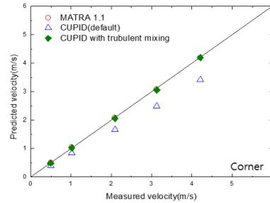
(a) Outlet velocity along axial direction (corner)
