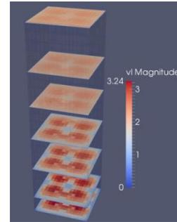
Fig. 9. Velocity contour with non-uniform inlet velocity
