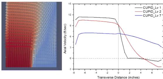
Fig. 13. Reverse flow occurrence at complete blockage case
