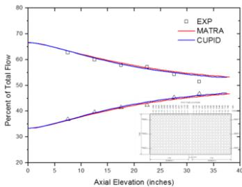
Fig. 11. Flow redistribution between two open rod bundles
