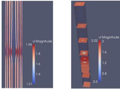
Fig. 6. Stream line and velocity contour along axial direction
