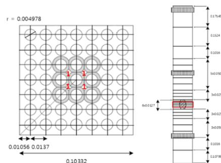
Fig. 5. Cross section and axial view of PNL 7x7 test section
