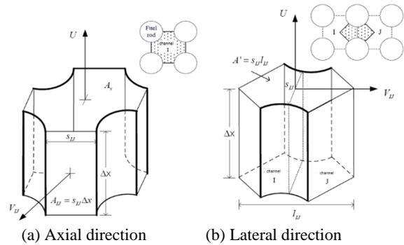
Fig. 1. Control volumes for subchannel governing equation
