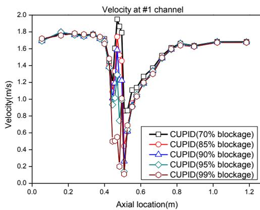
Fig. 8. Velocity with increasing of blockage ratio
