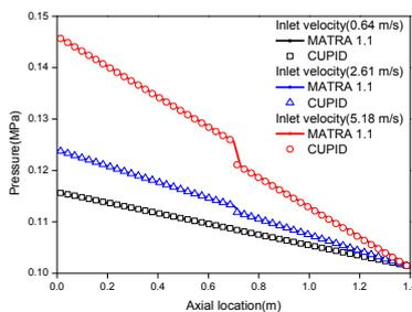
Fig. 3. Pressure drop along axial direction
