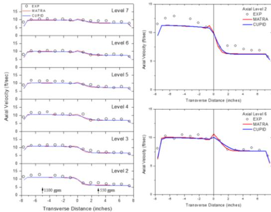
Fig. 12. Velocity distribution along axial direction at partial blockage case
