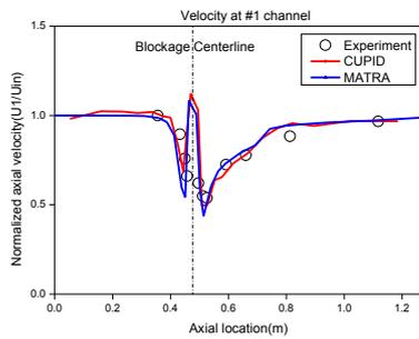
Fig. 7. Comparison results of the velocity at 70% blockage
