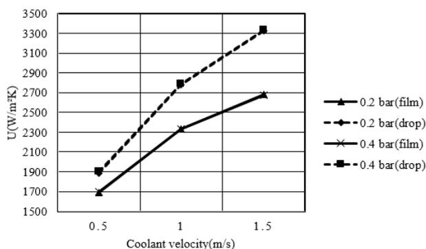
Fig 1. Overall heat transfer coefficient graph according to coolant velocity in conditions of 0.2 bar, 0.4 bar with filmwise & dropwise condensation.
