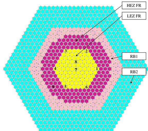
Fig. 1 Configuration of BFS-75-1 critical assembly
