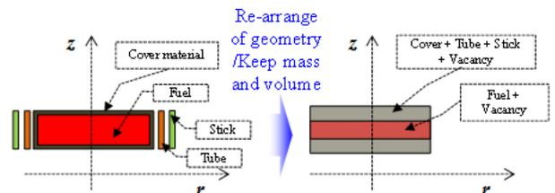
Fig. 4 Description of the 1-D homogenization method
