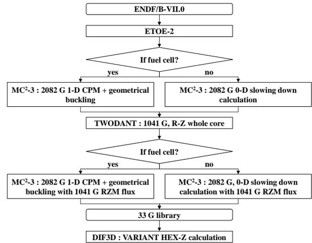
Fig. 2 MC<sup>2</sup>-3/DIF3D calculation procedure
