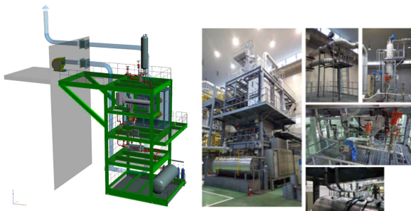
Fig. 1. The SELFA test facility (left:3D model, right:photos)
