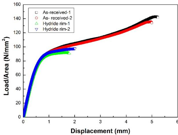
Fig. 3. Normalized load-displacement curve of Zircaloy-4 with hydride rim at room temperature.
