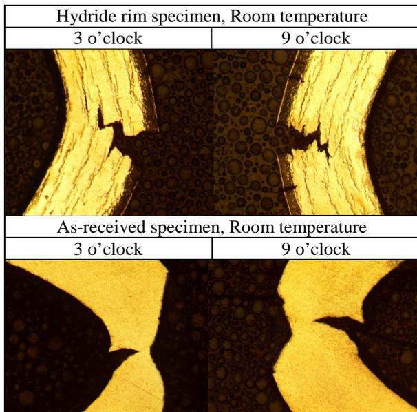
Fig. 4. Morphology and crack development in the specimen according to existence of hydride rim.
