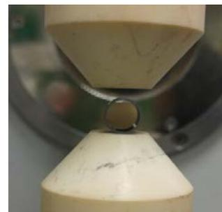
Fig. 2. Ring compression machine and sample.
