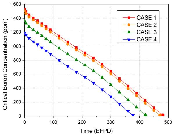
Fig. 4. Comparison of critical boron concentrations of 12<sup>th</sup> cycles for all cases
