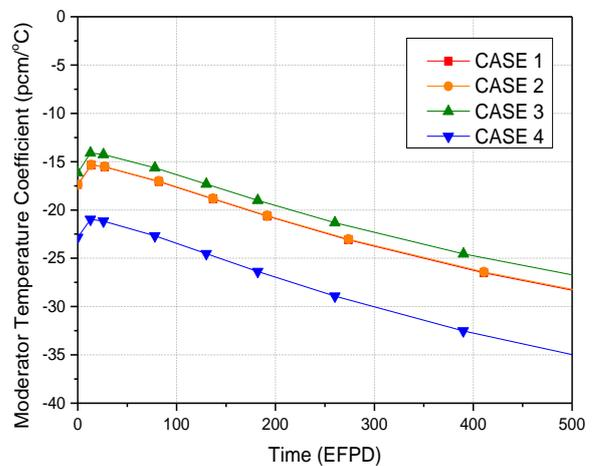
Fig. 11. Comparison of moderator temperature coefficients of the fuel assemblies having different fuels
