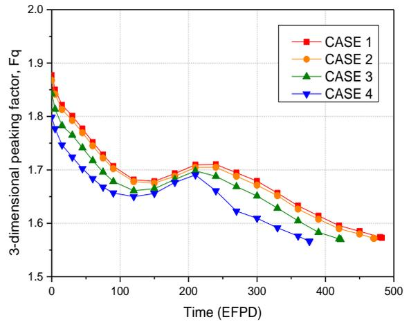
Fig. 6. Comparison of 3-dimensional peaking factors of 12<sup>th</sup> cycles for all cases
