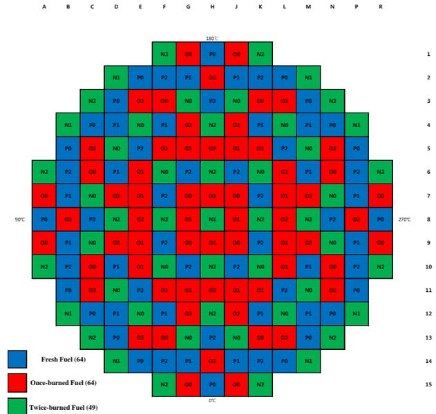
Fig. 3. Low-leakage loading pattern coupled with the concept of three batch refueling scheme of 12<sup>th</sup> cycle for all cases
