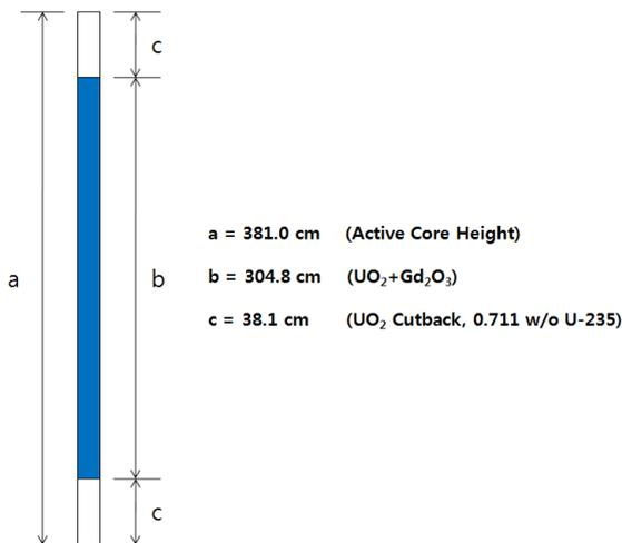
Fig. 2. Axial cutback configuration of burnable absorber rod
