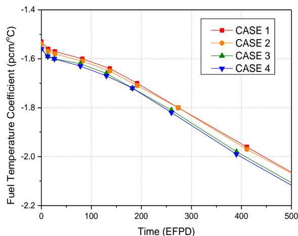
Fig. 13. Comparison of fuel temperature coefficients of the fuel assemblies having different fuels
