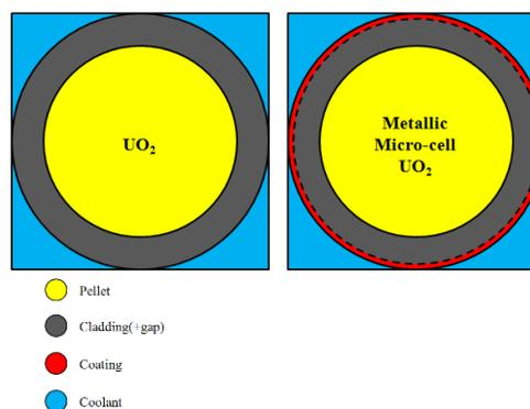
Fig. 1. Illustration of fuel pellet and cladding for reference fuel case and ATF cases
