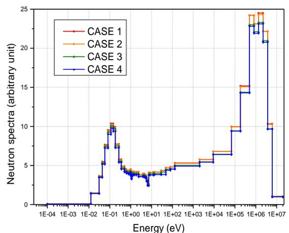
Fig. 12. Comparison of the neutron spectra of the fuel assemblies having different fuels
