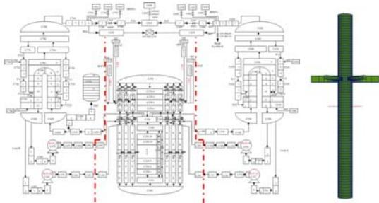
Fig. 2. 1-D Nodalization and 3-D RPV Mesh
