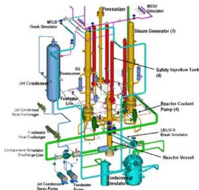
Fig. 2. Configuration of ATLAS Facilities [2]
