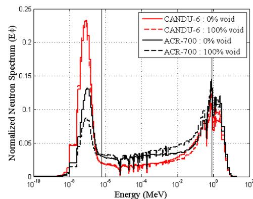
Fig. 1. Normalized neutron spectra at 0% and 100% coolant voiding.
