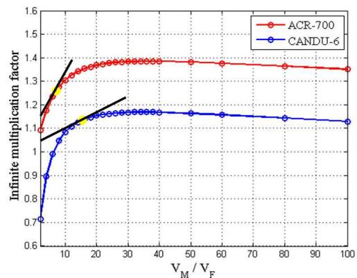
Fig. 3. Multiplication factor as function of the moderator to fuel volume ratio.
