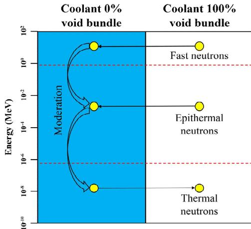
Fig. 2. Neutron behaviors upon checkerboard voiding.
