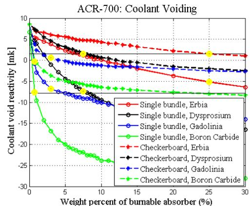
Fig. 7. CVR behaviors depending on BA materials upon single bundle and checkerboard voiding.
