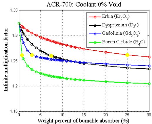
Fig. 6. Multiplication factor using various types of BA.
