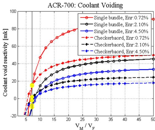
Fig. 5. CVR for variations of  $^{235}\text{U}$  enrichment upon single bundle and checkerboard coolant voiding.
