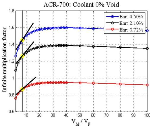
Fig. 4. Multiplication factor behavior for various enrichment of  $^{235}\text{U}$ .
