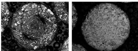
Fig.4. Cross section images of UO<sub>2</sub> kernel from washing and sintering condition change.
