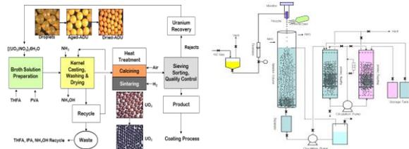
Fig. 1. A block diagram and experimental apparatus.
