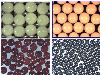
Fig.3. Photographs of liquid droplets, dried-ADU gel, UO<sub>3</sub> particles, and UO<sub>2</sub> kernel.
