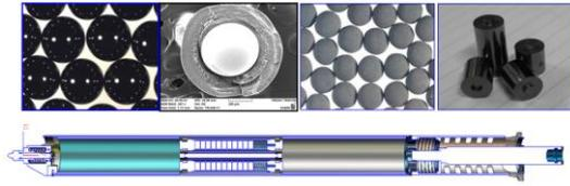
Fig.2. Photographs of kernel, TRISO, graphite compact, and irradiation test device.
