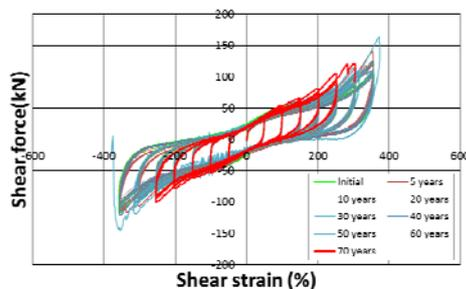
Fig. 4. Shear force and strain of LRBs with time
