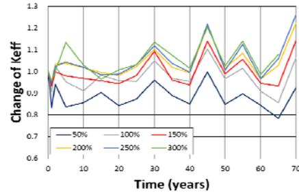
Fig. 5. The effective stiffness of LRBs with time
