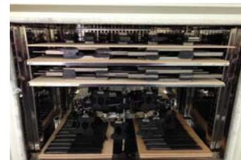
Fig. 2. Experimental setup for aging test of rubber
