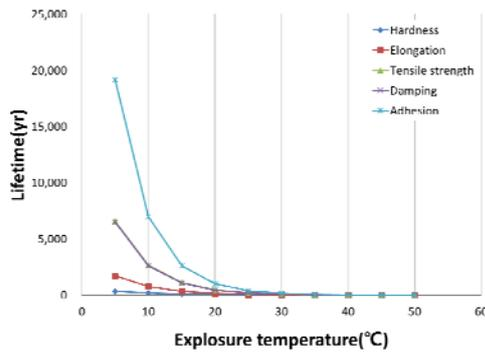
Fig. 3. Lifetime of rubber material at various temperature
