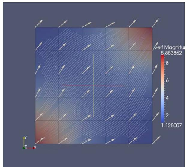
Fig.13. Liquid Velocity Field of original RELAP5 without cross flow
