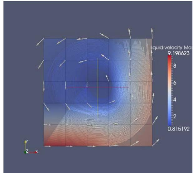
Fig.4. Liquid Velocity Field of Conservative RELAP5
