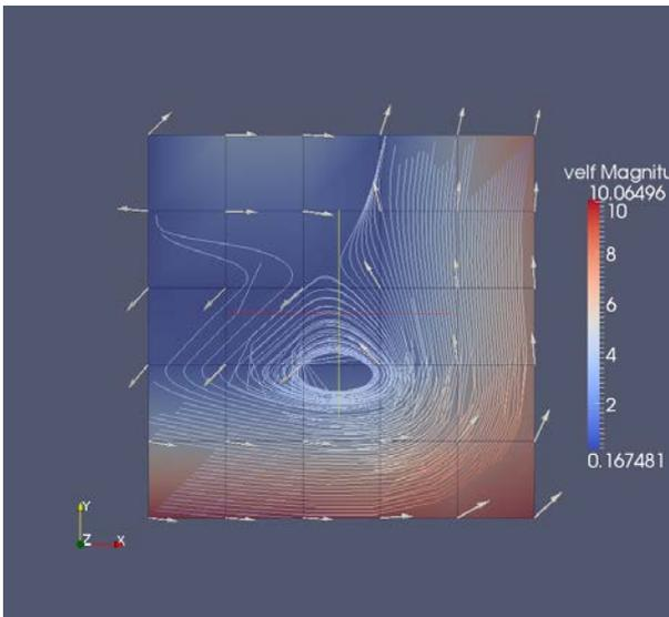
Fig.11. Liquid Velocity Field of original RELAP5 with cross flow
