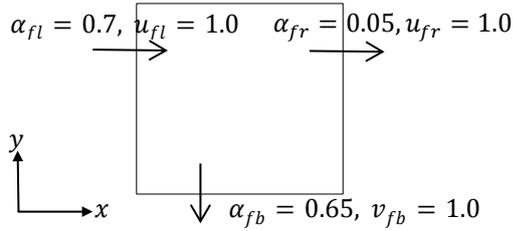
Fig.1. Flow Configuration of a Cell
