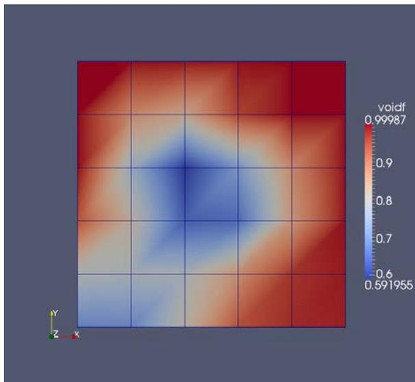
Fig.3. Liquid Fraction of Conservative RELAP5
