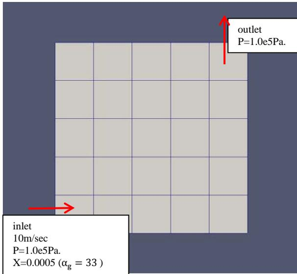
Fig.2. 5x5 2-dimensional Flow Test Simulation
