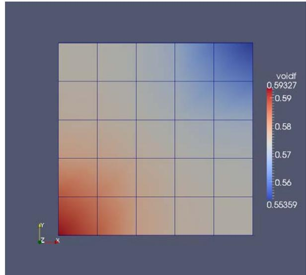
Fig.12. Liquid Fraction of original RELAP5 without cross flow
