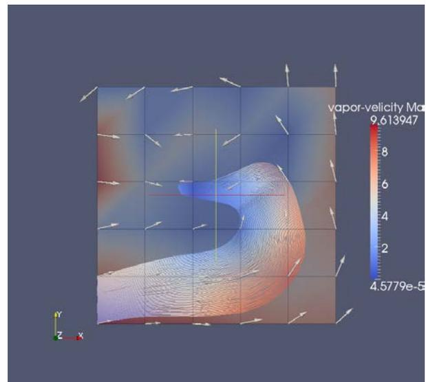
Fig.5. Vapor Velocity Field of Conservative RELAP5
