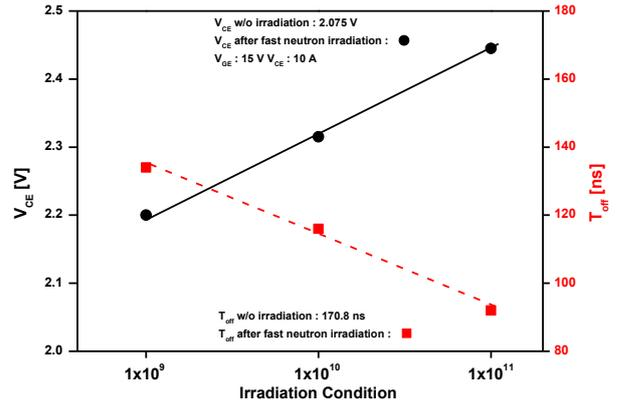
Fig. 6 On-state forward voltage drop of the IGBT
