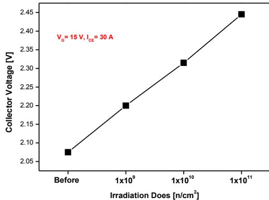
Fig. 4 On-state forward voltage drop of the IGBT
