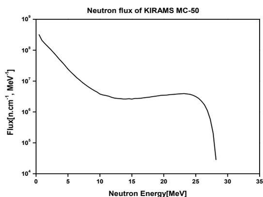
Fig. 2 Neutron spectrum generated by the <sup>9</sup>Be(p,n) reaction in the MC-50 cyclotron
