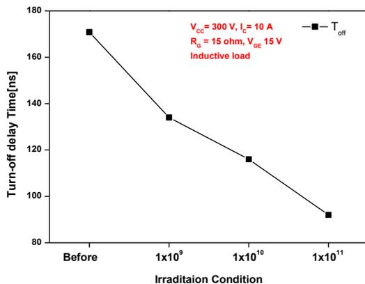
Fig. 5 Turn-off delay time of the IGBT
