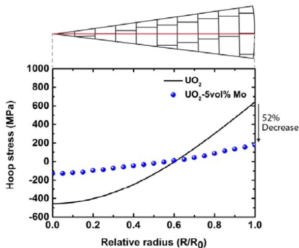
Figure 3. Hoop stress distributions of  $\text{UO}_2$  and  $\text{UO}_2$ -5 vol% Mo micro cell pellet.
