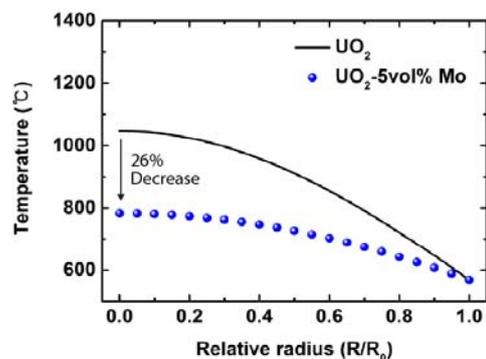
Figure 2. Comparison of temperature distributions between  $\text{UO}_2$  and  $\text{UO}_2$ -5 vol% Mo micro cell pellets.
