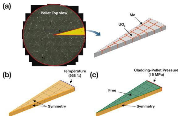
Figure 1. (a) Optical image (left) and 3D simulation model (right) of  $\text{UO}_2$ -5 vol% Mo micro-cell pellet. (b) Thermal boundary conditions of 3D simulation model. (c) Mechanical boundary conditions of 3D simulation model.
