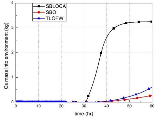
Fig. 4 Cs mass into environment from containment during 60 hours after each accident
