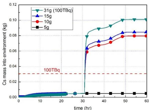
Fig 6. Cs mass during 60 hours after SBLOCA with different starting time of spraying
