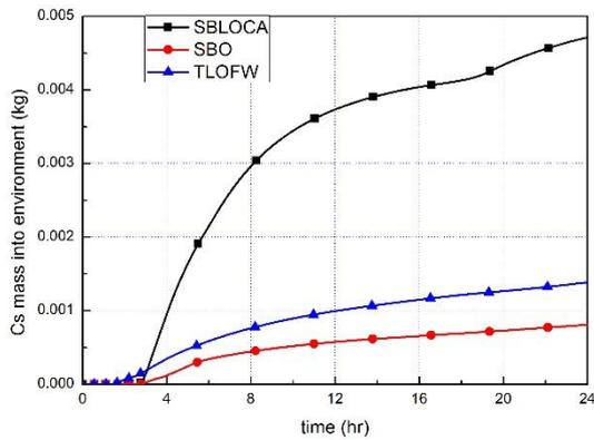
Fig. 3 Cs mass into environment from containment during 24 hours after each accident
