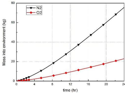
Fig. 2 Released air into environment from containment by leakage of defects following time
