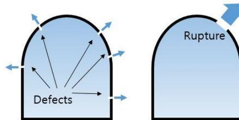
Fig.1 Diagram of leakage by defect (left) and leakage by rupture (right) in containment
