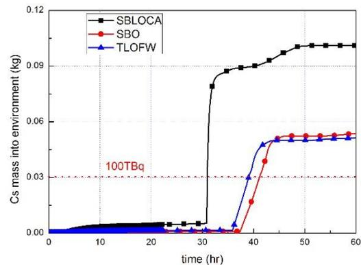
Fig. 5 Cs mass into environment from containment during 60 hours after each accident with CSS
