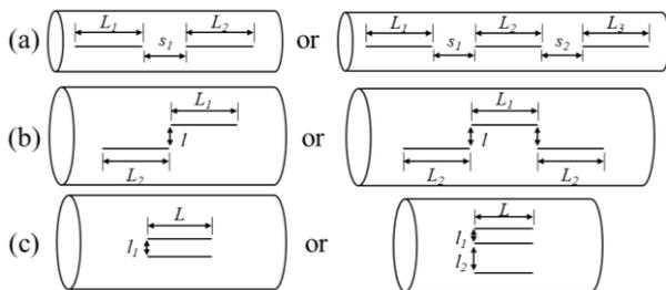
Fig. 1. Shape of multiple flaws: (a) Collinear axial flaws, (b) Non-aligned axial flaws, (c) Parallel axial flaws.
