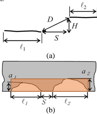
Fig. 2. Shape of multiple flaws: (a) non-aligned flaws, (b) coplanar flaws.
