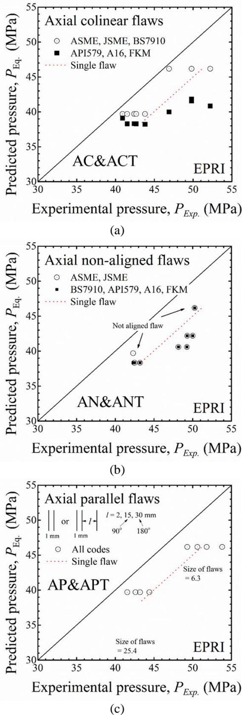
Fig. 3. Comparison of predicted result with experimental data: (a) axial collinear flaws, (b) axial non-aligned flaws, (c) axial parallel flaws.
