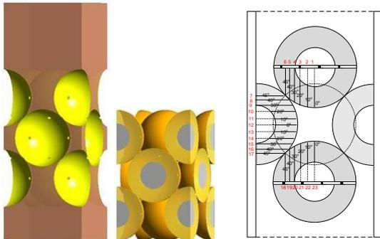
Fig. 1 The fluid part (left) and solid part (middle) and locations of temperature measuring point in plane 1(right).
