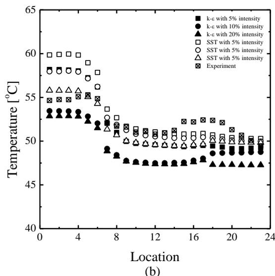
Fig. 3 (a) comparison of simulation and experiment results with pebbles contact diameter of 6mm and (b) of 3.5mm
