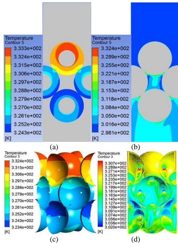
Fig. 2 (a) the pebbles' temperature profile in plane 1
