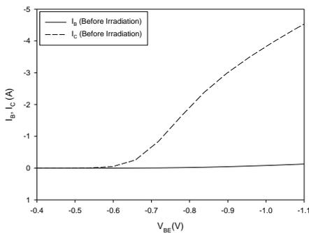
Fig. 2. Base and collector currents versus base-emitter voltage for before fast neutron irradiation.
