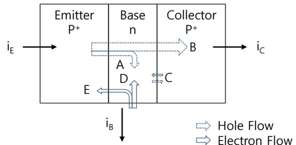
Fig. 1. Hole and electron flows in a p-n-p BJT with forward-biased emitter junction and reversed-biased collector junction.
