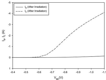
Fig. 3. Base and collector currents versus base-emitter voltage for after fast neutron irradiation.
