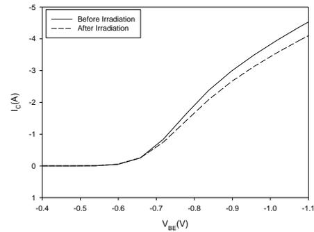
Fig. 5. Collector currents versus base-emitter voltage for before and after fast neutron irradiation.
