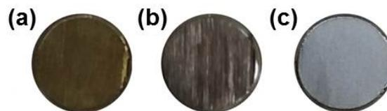
Fig. 1. Optical images of U-10Zr samples (a) before and after the heating at (b) 610 and (c) 1130 °C.
