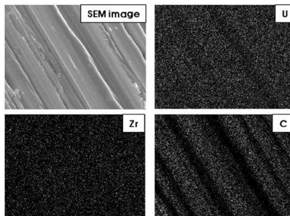
Fig. 2. SEM image ( $\times 3,000$ ) and EDS mapping data of uranium, zirconium, and carbon elements obtained from U-10Zr sample before the heating.
