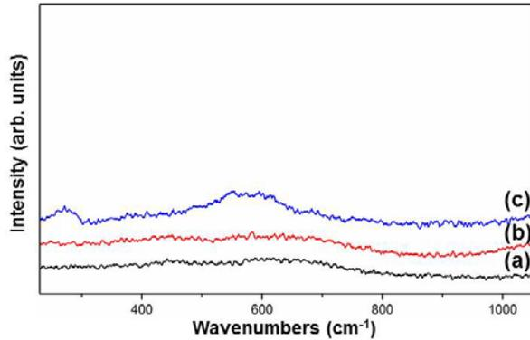
Fig. 3. Raman spectrum of U-10Zr samples obtained in range of 230 to 1050 cm<sup>-1</sup> (a) before and after the heating at (b) 610 and (c) 1130 °C.
