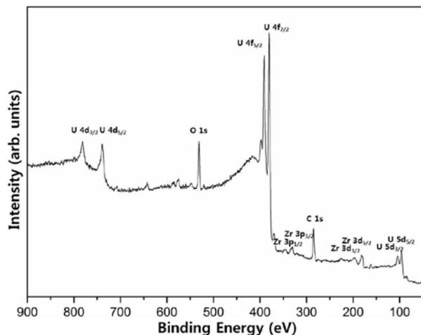
Fig. 4. XPS survey spectra of U-10Zr sample after the heating at 1130 °C.
