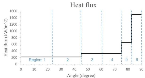
Fig. 2. Heat flux distribution of reactor vessel lower head
