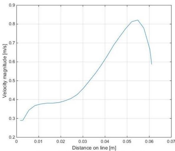
Fig. 5. Velocity profile of air-water flow,  $500 \text{ kg/m}^2\cdot\text{sec}$  case.
