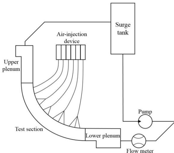
Fig. 1. Schematic diagram of flow measurement loop
