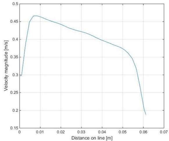
Fig. 4. Velocity profile of water flow, 400 kg/m<sup>2</sup>·sec case.
