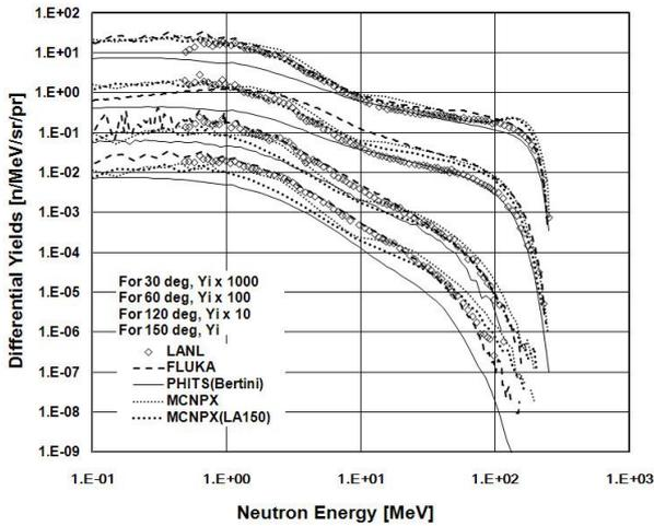
Fig. 1. Differential neutron yields from thick iron targets irradiated by protons of 52 MeV (upper), 113 MeV (Middle), and 256 MeV (Lower).
