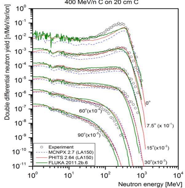
Fig. 2. Differential neutron yields from thick carbon targets irradiated by carbon beam of 100 MeV/n (upper), 180 MeV/n (Middle), and 400 MeV/n (Lower).
