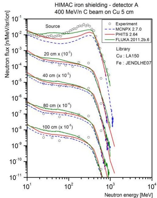
Fig. 4. Neutron spectra behind of each panel of 20 cm-thick iron shield when neutrons are produced from 5 cm Cu target irradiated by 400 MeV/n Carbon.
