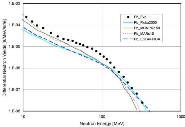
Fig. 3. Differential neutron yields from thick Pb target irradiated by electrons of 2.5 GeV.
