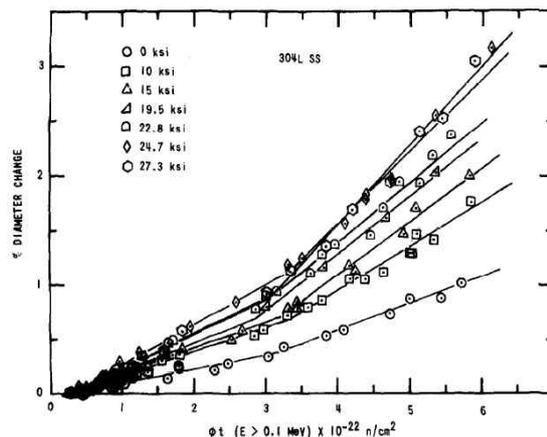
Composite of all diameter changes vs fluence data from the Type 304L stainless steel creep experiment.
