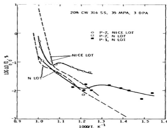
Figure 3. Temperature dependence of irradiation creep for 316CW, relative to thermal creep
