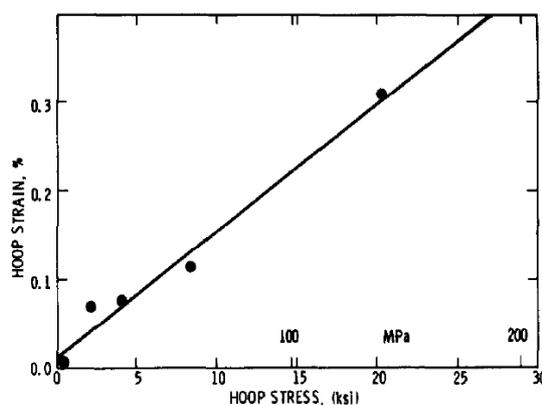
Stress dependence of irradiation creep 20% CW Type 316 stainless steel 520°C -  $3 \times 10^{22}$  n/cm<sup>2</sup>.
