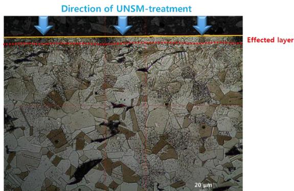
Fig. 3. Cross-sectional OM image of UNSM-treated STS316L.
