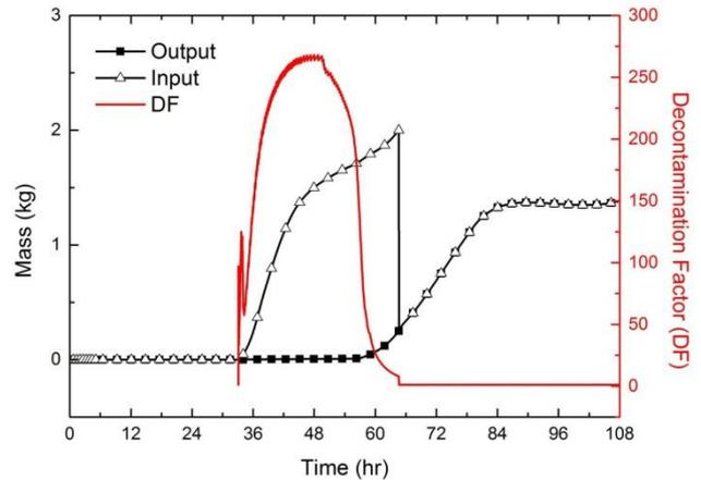
Fig. 3. Decontamination factor calculated by input and output of CsI aerosol mass on scrubbing solution [2].
