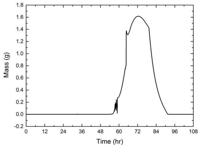
Fig. 2. Accumulated mass of CsI aerosol in the FCVS vessel atmosphere [2].
