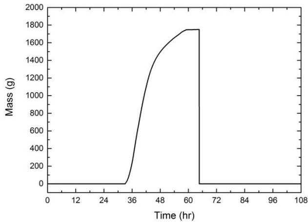
Fig. 1. Accumulated mass of CsI aerosol in a pool in the FCVS vessel [2].
