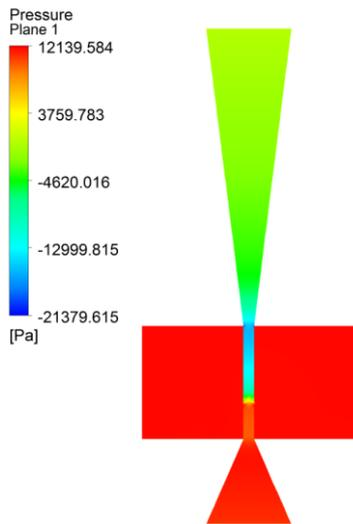
Fig. 3 Pressure Contour in Venturi Scrubber
