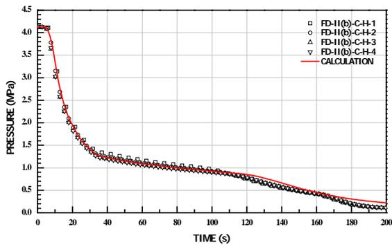
Fig. 4. Calculation Result of VAPER Test - Pressure
