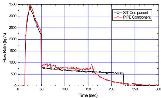
Fig. 9. Comparison of SIT Discharge Flow Rate
