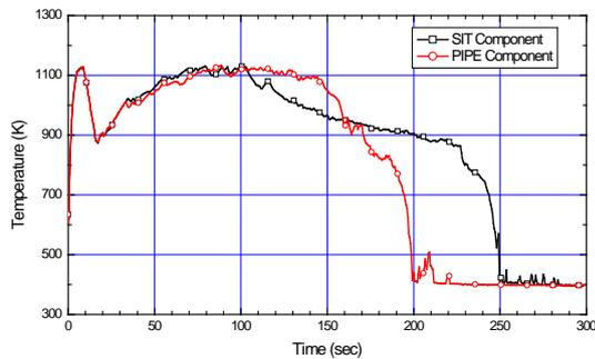
Fig. 10. Comparison of Cladding Temperature at PCT Node
