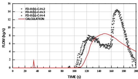
Fig. 5. Calculation Result of VAPER Test - Gas Flow Rate
