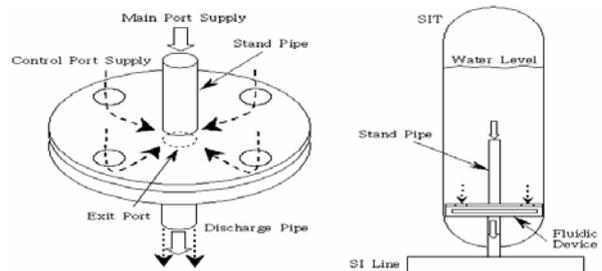
Fig. 1. Schematic Diagram of FD-SIT
