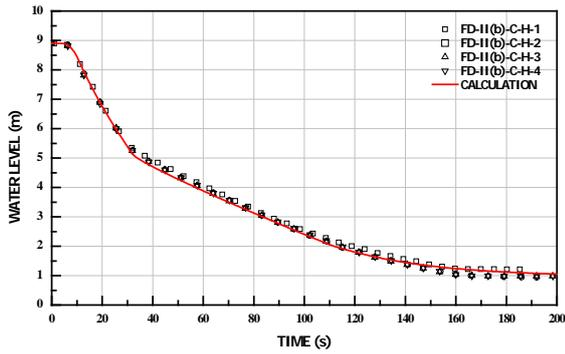
Fig. 3. Calculation Result of VAPER Test - Water Level
