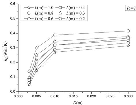
Fig. 4.  $h_h$  according to the diameter of vertical pipe( $Pr=7$ ).
