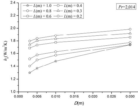
Fig. 3.  $h_h$  according to the diameter of vertical pipe( $Pr=2,014$ ).
