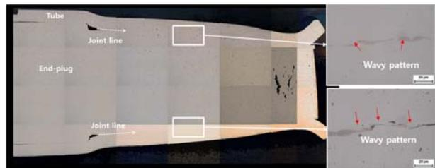
Fig. 5. Optical micrograph of the longitudinal section of MPWed sample.
