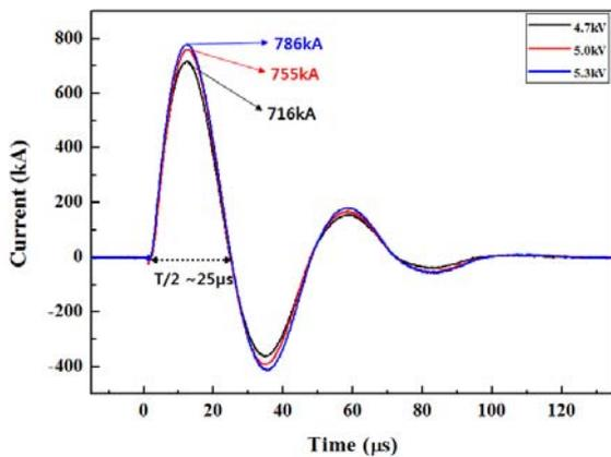
Fig. 3 Typical oscillating current wave form after pulse.
