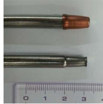
Fig. 4. External appearance of MPWed HT9 steel tube samples; the copper driver sleeve shown on the upper sample was removed from the lower sample.
