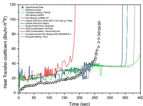
Figure 6. Sensitivity result for wall heat transfer correlations
