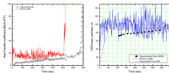
Figure 2. Reflood HTC and CRF for test number of 0690
