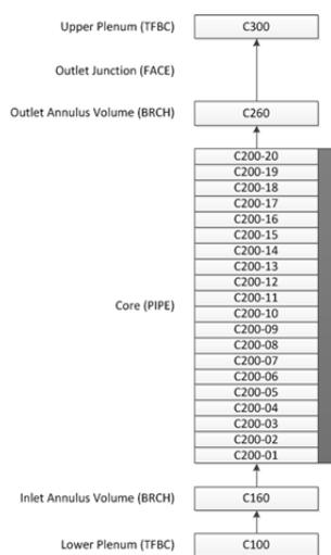
Figure 1. Modeling using SPACE for FLECHT Test
