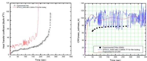
Figure 7. Reflood HTC and CRF for test number of 6948 with COBRA-TF film boiling correlation
