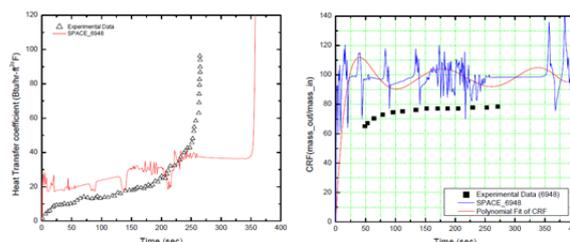
Figure 5. Reflood HTC and CRF for test number of 6948
