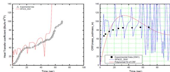
Figure 3. Reflood HTC and CRF for test number of 3541
